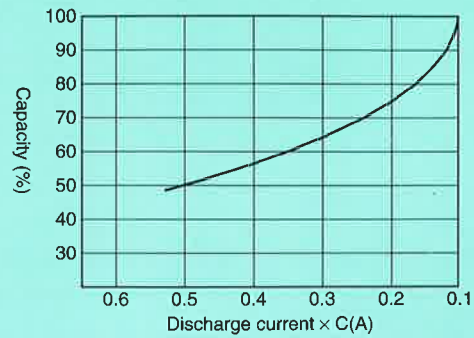
CS type discharge current-capacity characteristics
