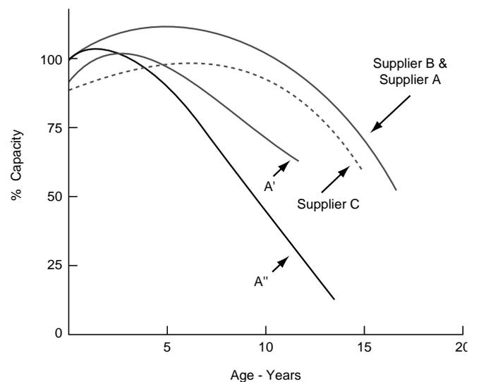
Fig. 1 Aging Characteristics of 180-1680 Ah Pb-Ca Batteries
