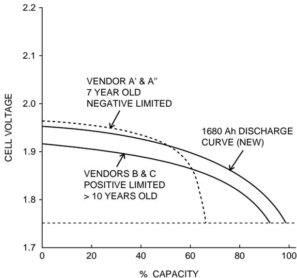
Fig. 2 Discharge Characteristics of 1680 Ah Pb-Ca Batteries After Aging
