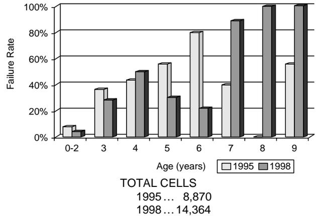
Fig. 7: Cell Failure Data-1995 Versus 1998 Results [14]
