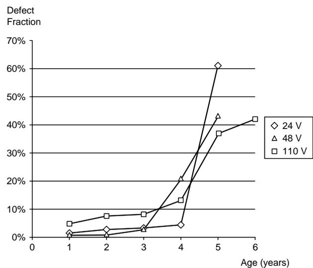
Fig. 8: Battery Defect Fraction(Fig. 1 of INTELEC Paper [26])
