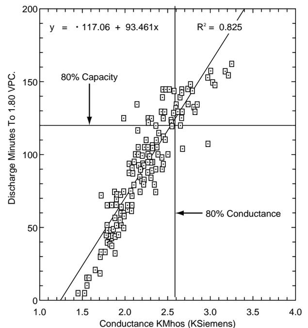
Fig. 9 Discharge Capacity vs Conductance. VRLA 1000 Ah. 168 Cells Consolidated Date (Strings 9-15). 263 Amps. To 1.80 Volts Per Cell.
