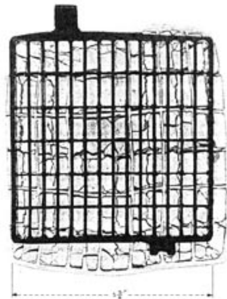
図1 初期形状と腐食後の正極格子基板形状 Fig.1 Corroded positive plate with original grid overlaid to initial dimensions.
