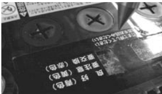
図8 静電気印加試験 Fig.8 Static electricity test
