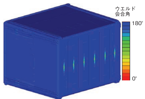
図4 電槽成型時のウエルド会合角解析結果 Fig.4 Calculation result of resin meeting angle during battery container forming
